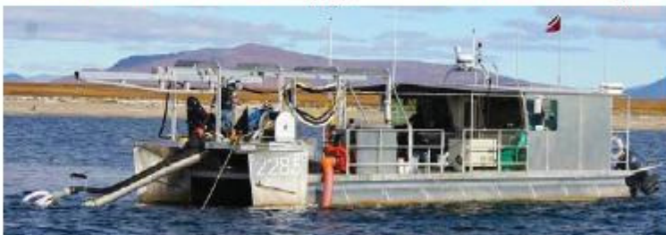
The 60' long "Havilah" is our primary 10" diver operated suction dredge for gold recovery. It is designed to mine continuously when dredging conditions are favorable.
